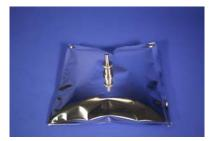
Multi-Layer Foil bags provide light and moisture protection for low molecular weight compounds such as hydrogen that are unstable when collected into standard Tedlar® bags. Use a low flow air sample pump with exhaust port.
